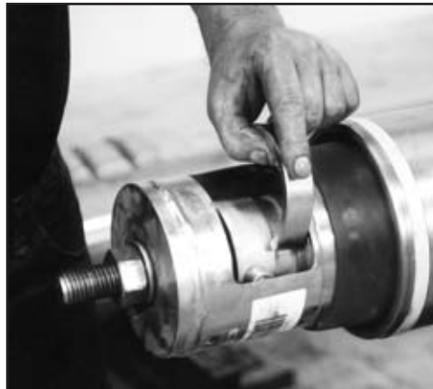
FIG. 129: INSTALL SEGMENT RING
