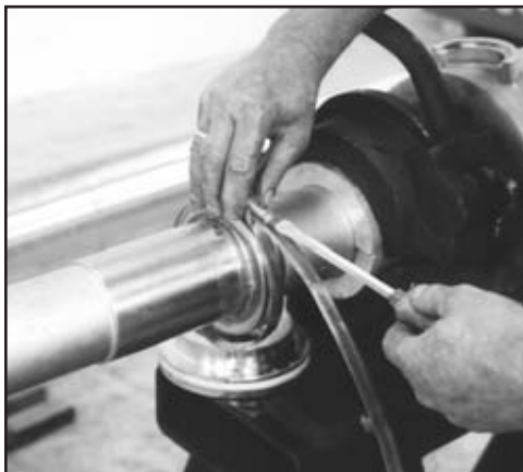
FIG. 119: USE COMPRESSION CLAMP TO REFORM SEAL
