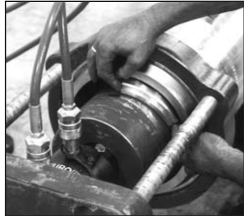
FIG. 131: INSTALL SEGMENT RING
