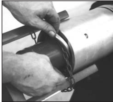
FIG. 79: INSTALL SEGMENT RING
