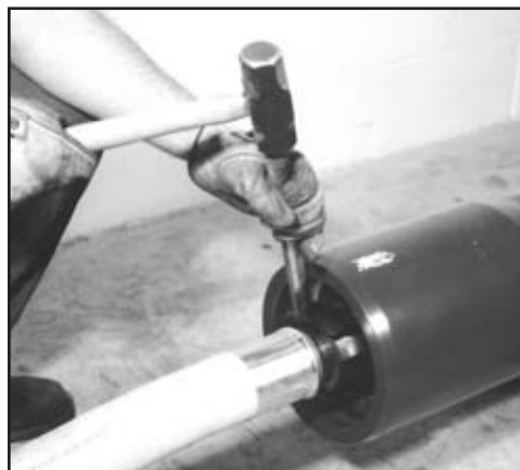
FIG. 60: REMOVE OLD AIR HOSE AND REPLACE WITH NEW ONE
