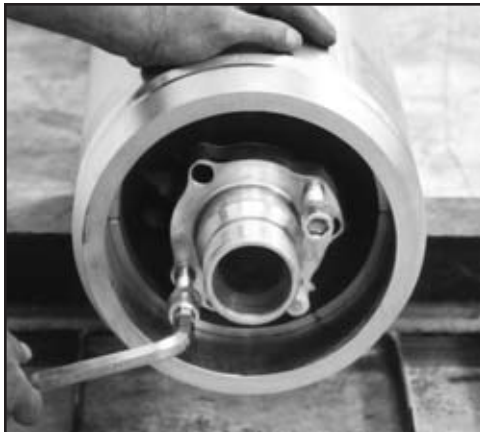
FIG. 86: USE TWO SET SCREWS AS JACK SCREWS
